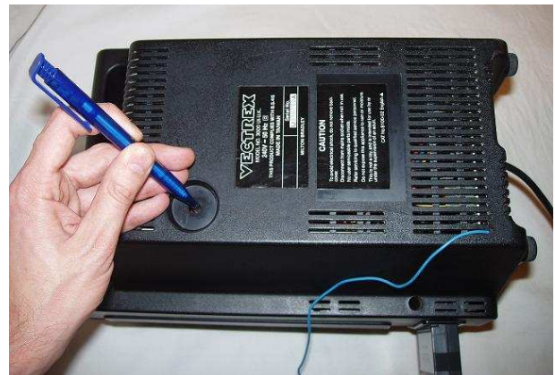
Fig. 4 Using a pen to “pull” the brightness shaft into the correct position
