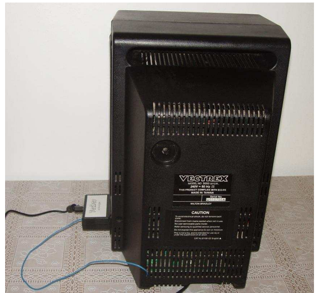
Fig. 5 VecDev cartridge and reset signal incorporated with Vectrex console
